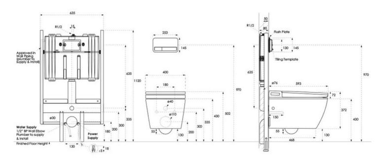
Note: All dimensions are in millimetres and are subject to normal manufacturing variations. Always use the physical product measurements for cut-outs and rough-ins as the technical details shown may differ from the actual product. Use acetic cured silicone sealant. Do not use epoxy type adhesives. Clean with damp cloth. Do not use abrasive cleaners, liquids or pastes.
