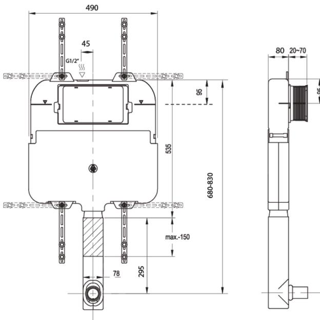
The slim concealed, dual flush cistern is made from high density polyethylene, incorporating inbuilt overflow. Due to its slim design, the cistern can be installed in a standard 90mm metal or timber stud wall application.
