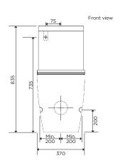
The Synergii suite is a stylish and functional back to wall toilet suite. It has a rimless bowl eliminating the conventional box rim making this toilet very hygienic and easy cleaning. It's fitted with a soft close Haro seat, so one touch and it closes gently and quietly.
