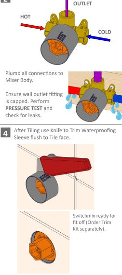
before performing pressure test. FOR STANDARD PRESSURE TESTING 八 Up To 500Kpa Test Plug Test Cap
