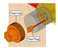
For high pressure testing of pipes, remove Test Cap and add another Test Plug into the Cold Inlet.
