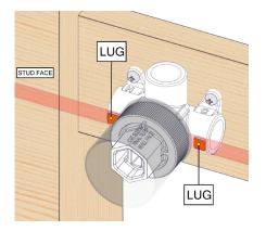
Check Lugs (Highlighted in ORANGE) are Flush with Front of Stud.
