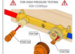
For high pressure testing of pipes, remove Test Cap and add another Test Plug into the Cold Inlet.
