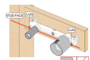
Screw the Mixer Breach onto Nogging to dimensions shown in adjustment
