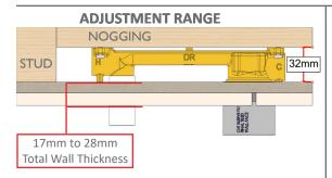
Range from the Nogging face to the Stud Face is 32mm as shown.
