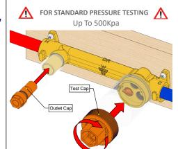
SwitchMix comes pre-installed with a Test Plug in the Hot Inlet only and a Test Cap.
