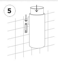
Slide toilet roll holder down onto the bracket. Re-insert inner sleeve and toilet brush.
