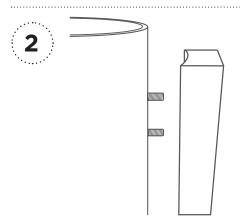
Feed x2 10mm screws into holes with the head of the screw inside of the holder.
