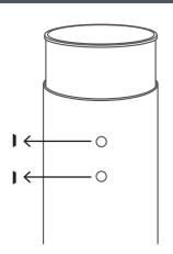
Attach the wall bracket securely to the wall in the desired location (making sure it is straight). Ensure the flat part of the bracket is against the wall.
