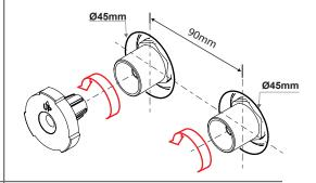
5 Fit Spindle Sleeve over the spindle adaptor.
