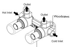
Note: Do not remove | Protective cover protective covers until final fit-off.
