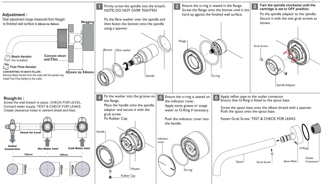
recommended working pressure 150-500KPa maximum hot water temperature 75 degrees
