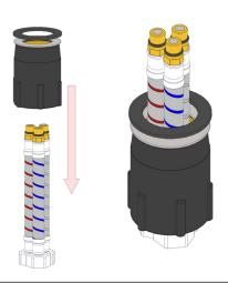
Slide Mixer Body through Benchtop hole and screw Locknut in place.
