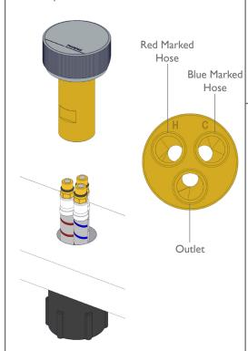
Feed Hoses through the bottom end of the Locknut and both Washers.
