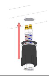
Connect Marked Blue & Red Hoses to wall Outlets and connect Plain Hose to Chosen Hob Outlet.
