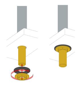
2 Slide Dress Plate and O-Ring onto Threaded Tail. Then slide Outlet Body through 25mm benchtop hole.
