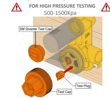
For high pressure testing of pipes, remove Test Cap and add another Test Plug into the Cold Inlet. Re-attach Test Cap. Hand Tighten + 120° OR 10 N m.
